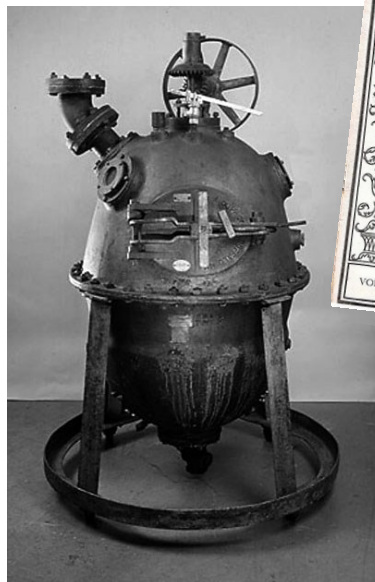
The Bakelizer applied heat and pressure to “bake” or harden the material
